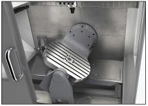
The UMC-750SS's high-speed trunnion table offers 150 deg/sec rapids to quickly position
