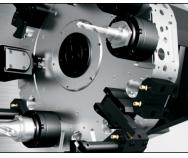
Dual-spindle turning combined with Y axis, C axis, and high-torque 6000-rpm live tooling allow multiple operations in a single setup to reduce part handling and increase accuracy.
